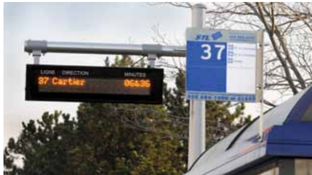
Digital display at a stop on route 37, on avenue Francis-Hughes, showing the waiting time before the next two buses arrive, in real time.
